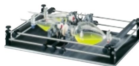
3 3 Rack systems Combifix SM, assembly C No. 0050 156
