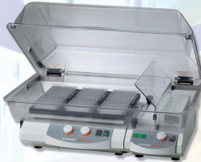
Application sample: Titramax 1000 + heating module + flat hood
