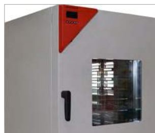
Viewing window in the door
