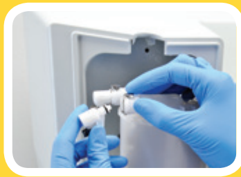
Quick-connect design allows for easy cartridge change-outs.
