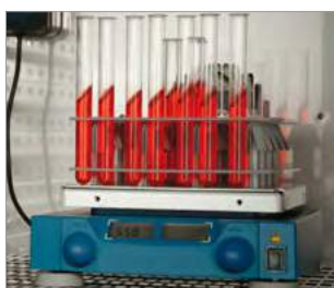
Shaker operation in the chamber
