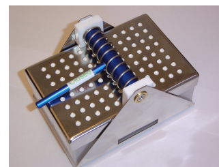
Fig 2. Sandwich covers convert all individual wells of square deepwell plates into 96 'mini-reactors'
