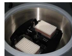
Figure 3. The Cryobank vials and rack were exposed to repeated and extensive centrifugation. No observations of either stress lines or deformities of the vials were observed.
