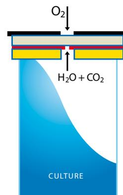
Cross-section of Micro-Flask sandwich cover
